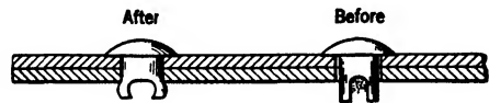
FIGURE 345. Principle of explosive aluminum rivet, used chiefly in locations not readily accessible for backing up.
